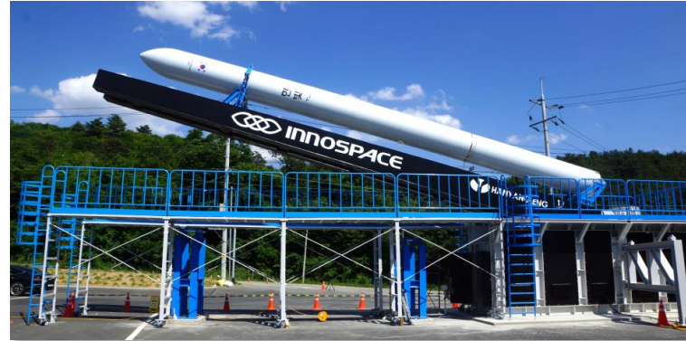
Launchpad with Erector
