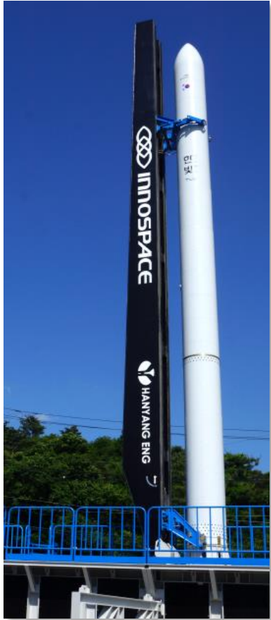
Erector Vertical Position
